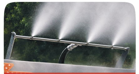
Anti-Smog Water Spray System
